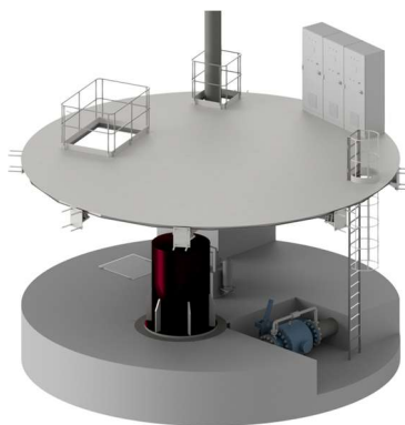
Fig. 7 Lower and upper levels of service platforms installed in the shaft
