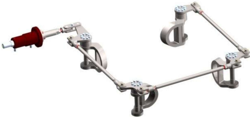
Fig. 9. Jet deflector (symbolic picture of 4-nozzle unit) [1].
