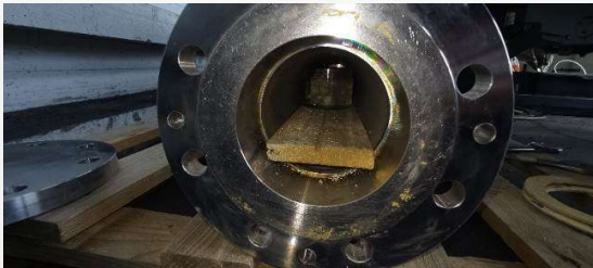
Stand for testing the corrosion of construction materials in the presence of CO 2 under pressure
