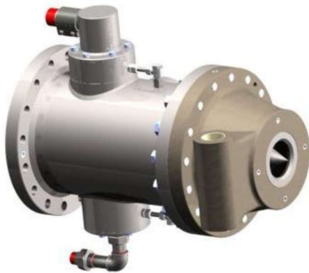
Fig. 11. Needle-type regulating nozzle for a Pelton turbine
