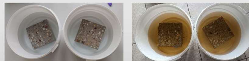
Leaching performance at the beginning and after 180 days
