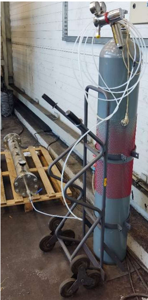
Stand for testing the corrosion of construction materials in the presence of CO 2 under pressure
