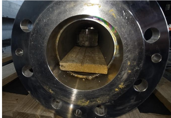
System for testing corrosion resistance under 6-bar CO 2 pressure.
