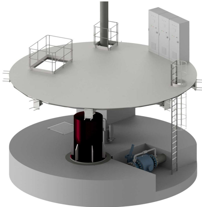
Fig. 26. Lower and upper levels of service platforms installed in the shaft [2].
