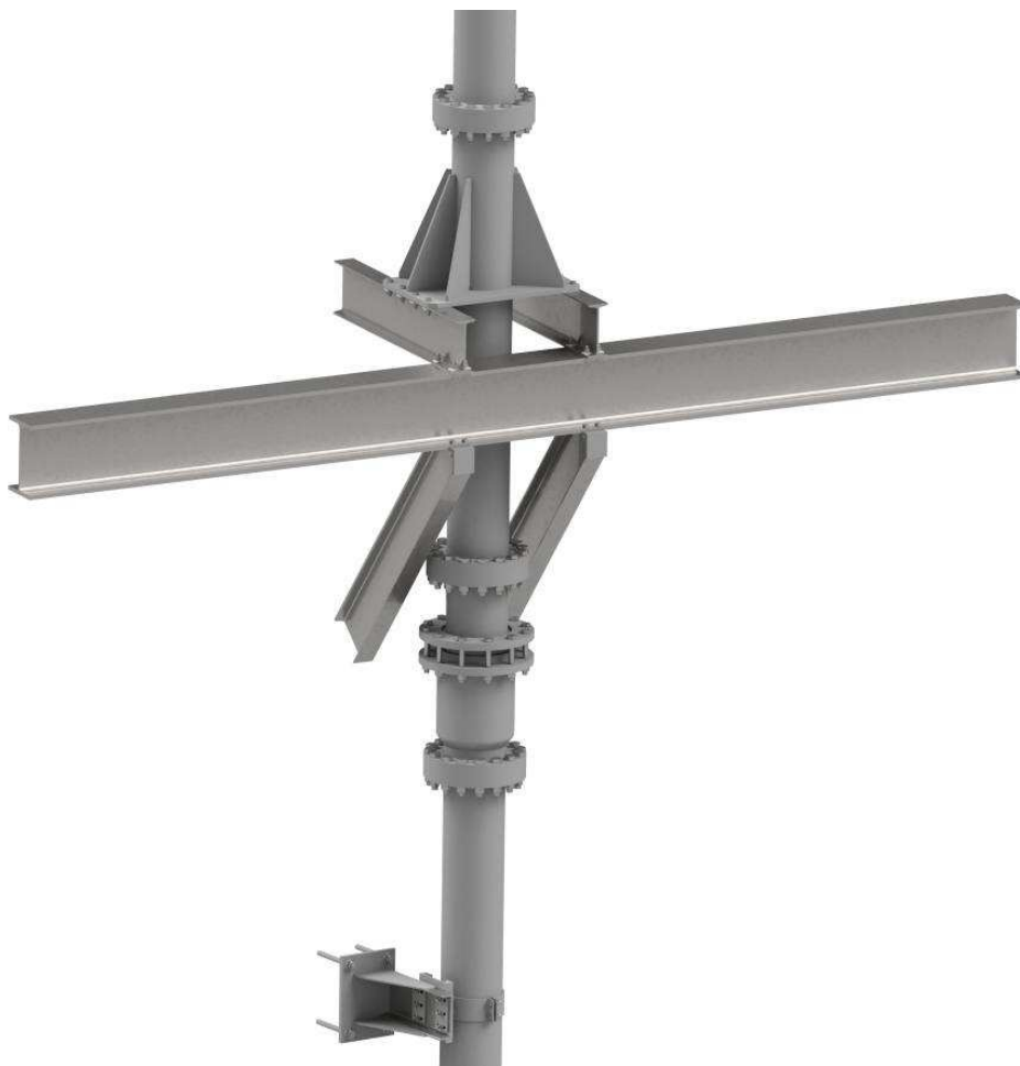
Fig. 15. Method of mounting the penstock on one of the supporting structures [2].
