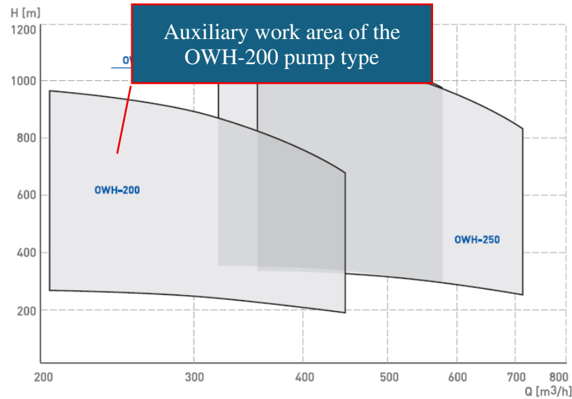
Fig. 42. Operating range of the OWH-200 pump [11]
