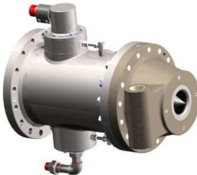
Fig. 11. Needle-type regulating nozzle [1].
