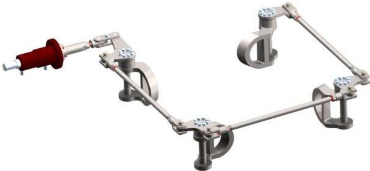
Fig. 12. Jet deflector (symbolic picture of 4-nozzle unit) [1].
