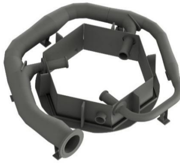
Fig. 31. Cross-section of the casing with a view of the turbine supply manifold
