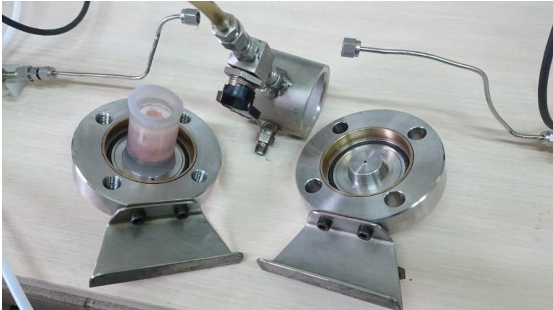
Figure 4 Holder during installation of a coated concrete sample.
